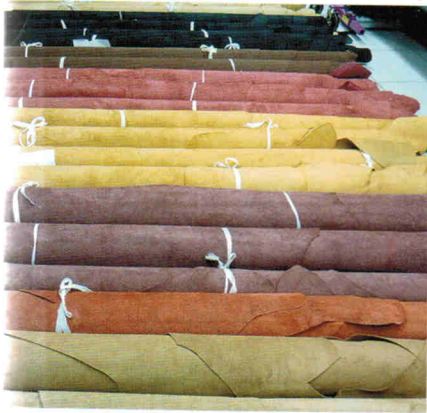
BELOW LEFT After vat or surface dyeing, cured Class Leather hides are wrapped up and prepared for shipping. BELOW RIGHT Modern-style coated leather utilizes fillers and spray-on vinyl finish for shiny, uniform appearance.
